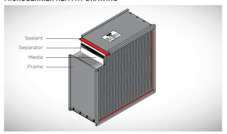
Microbarrier HEPA HT & HEPAMAX™ HT filters use a stainless steel frame that is bolted together for added strength and rigidity required for demanding environments where high temperature filters are utilized.
