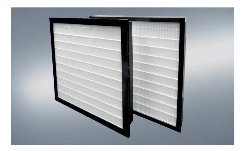
ULTRA 4 filters are designed utilizing a synthetic media in a minipleat configuration with a compact four inch deep plastic frame. The ULTRA 4 offers high efficiency (MERV 11, 13 and 14), a compact footprint, low resistance and many green benefits. The ULTRA 4 green benefits include a robust plastic frame as an alternative to metal or die-cut cardboard.
