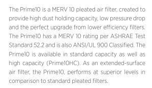
The Prime10 is the perfect upgrade from lower efficiency filters with the focus on fine particle removal as a result of the recent pandemic. The Prime10 offers MERV 10 high efficiency and low pressure drop making filter upgrades easy.
