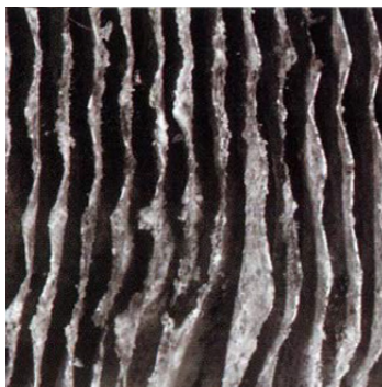
Coils treated with Tri-Kleen CP-XL after the same 4,000 hours.
