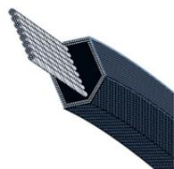
A variation of the classical belt, Hex belts come in AA, BB, CC or a deep CCP cross section. These belts transfer power from either side in serpentine drives. A drive design using Hex belts is more complicated and Continental's V-belt engineering manual should be consulted when replacing or troubleshooting these drives.
